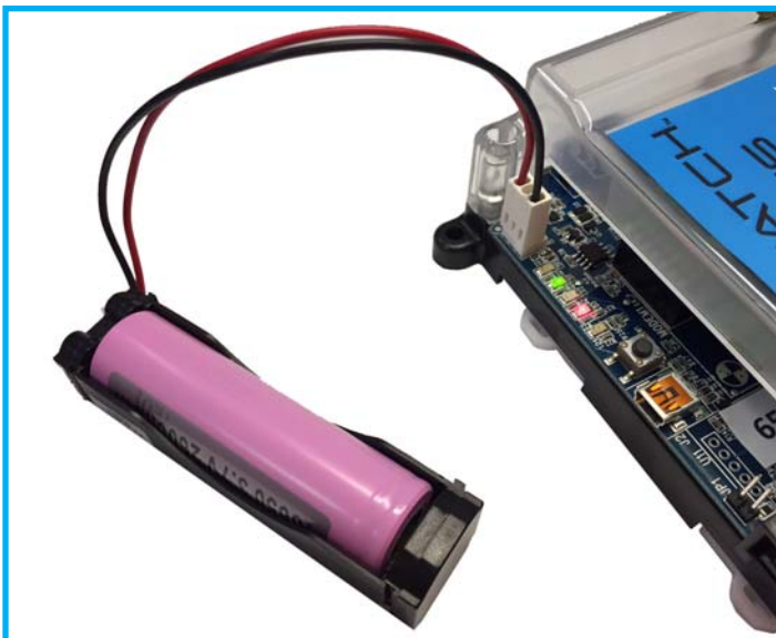
Backup Battery Connection
